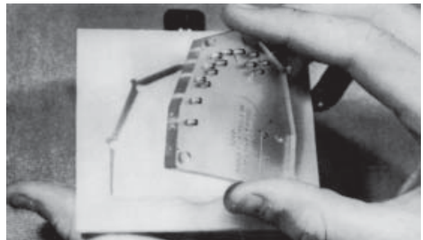
Plates with pins are inserted into the positioning matrix
